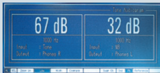
Large digits are preferred by some users and are therefore provided as an alternative to displaying audiograms.
